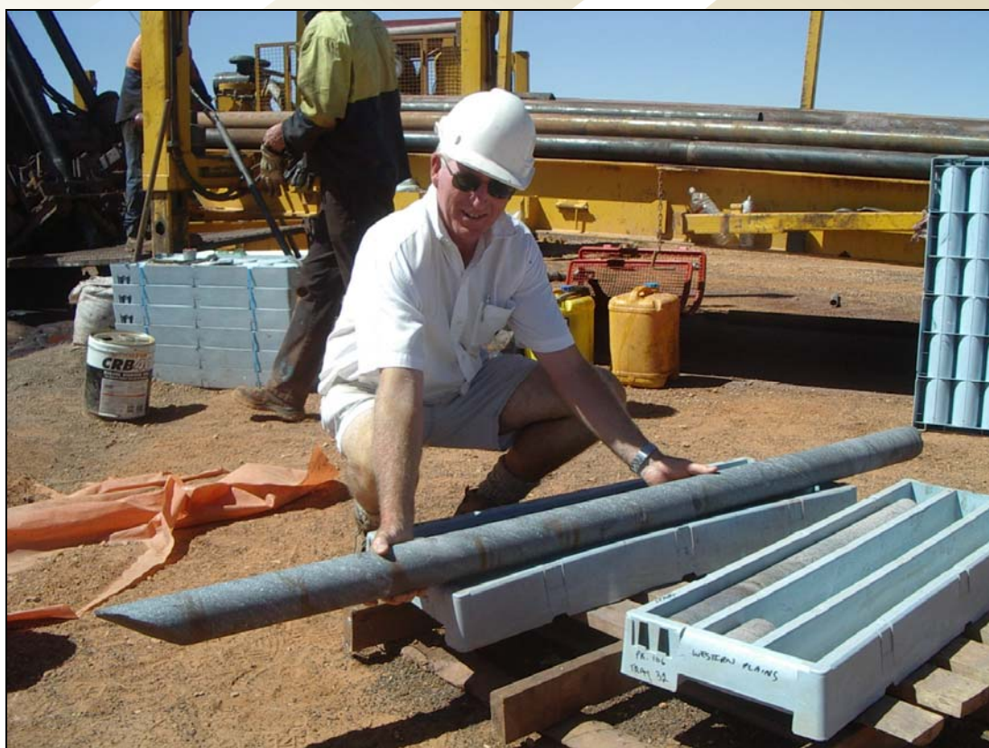
Figure 1 Massive High Grade Specular Haematite, PQ Core from Hole PK-107
